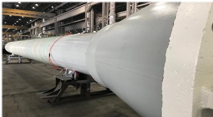
Figure 7. Cylinder casing (after coating repair).
